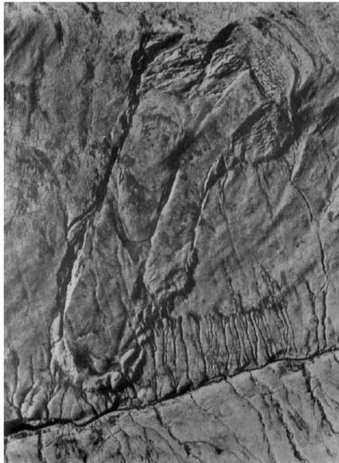
Figure 4. Vertical aerial photograph of the Fan Dringarth landslide. The headwall area lies near the top of the photograph. The length of the photograph represents about 1.2 km on the ground. © British Crown Copyright 1995/MOD. Reproduced with permission
