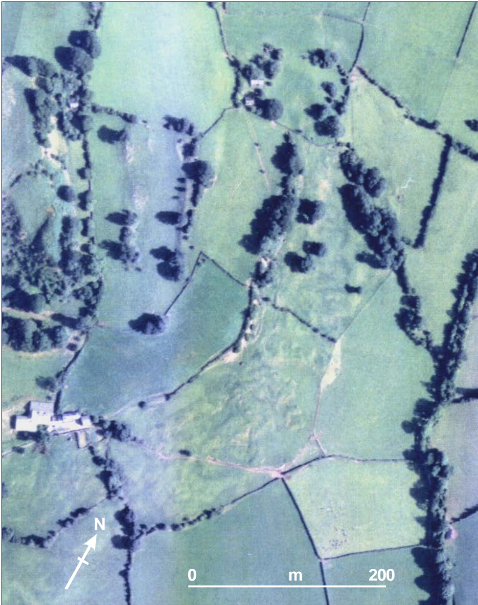
Shallow translational failures forming “hummocky ground” at Penywern Farm, Cwmyoy landslide Photograph: A. Humpage
