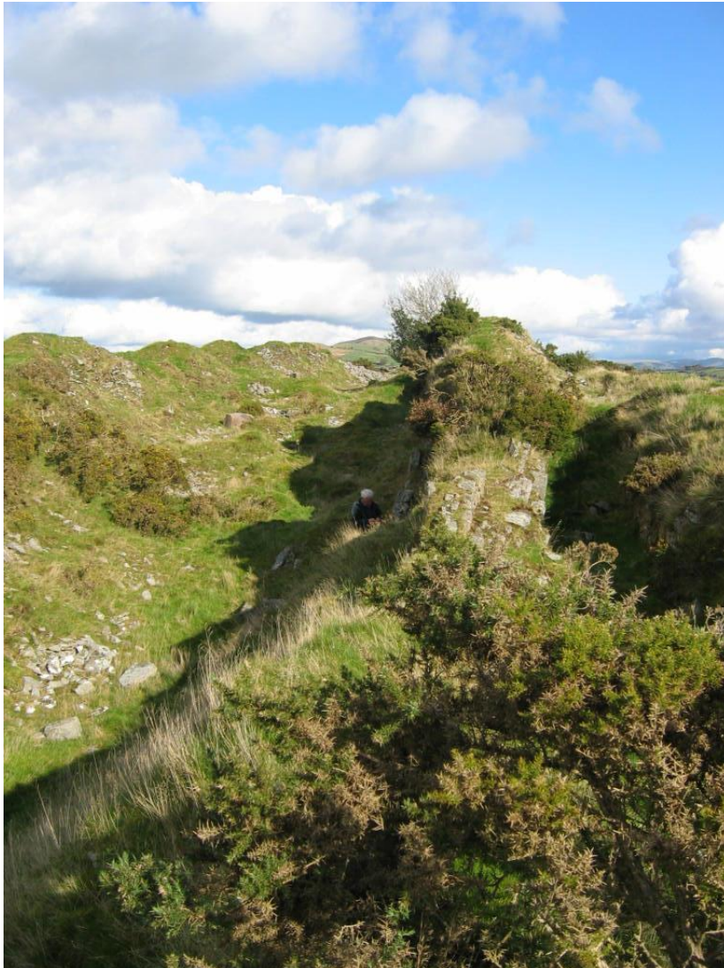
Tilestone crop working to left with unquarried ridge of coarse sandstone and conglomerate facies to right
