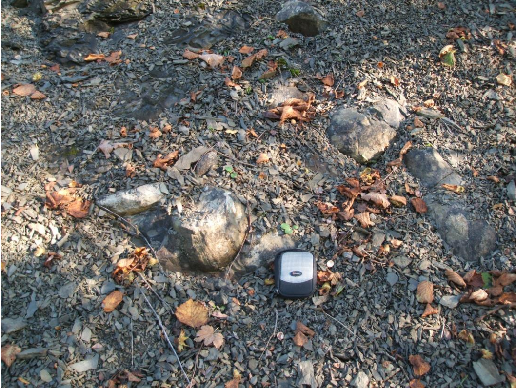
Figure 3. Close-up of randomly orientated calcareous nodules set in a structureless mudstone matrix within the Caer-beris Member, Builth Road cutting
