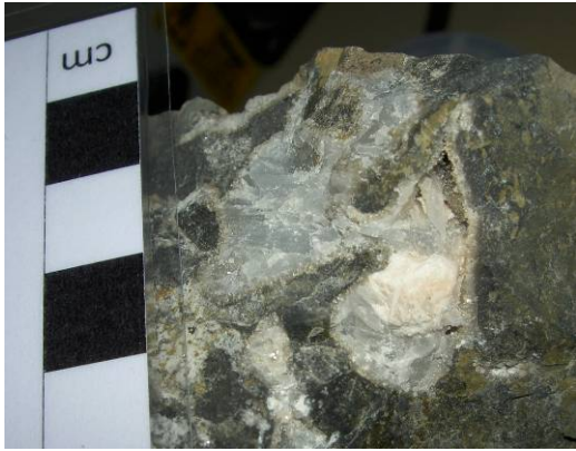
An example of interesting intergrowths not yet researched- celestine (blue) and gypsum (pink)
