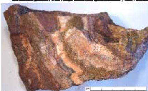
Ballinacraig Carboniferous limestone. Probably dolomite, pink calcite, pink limonite, goethite, minor limonite. Domes.
