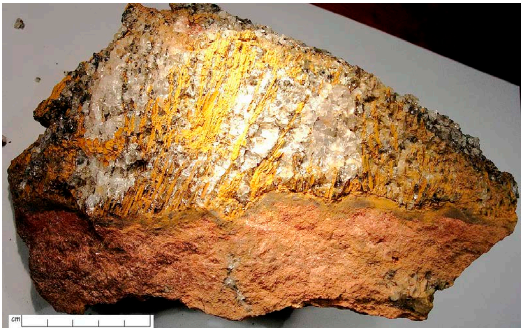
Iron mineralisation - large piece of brush type structure of quartz and goethite/limonite on Carboniferous Limestone - field of view 20cm across
