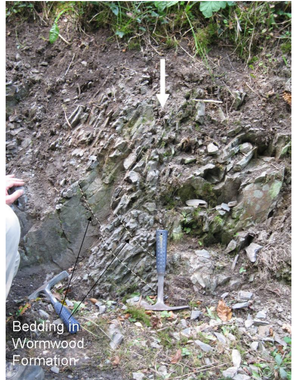
Photograph 2. Cefn Cerig road section; vertical slide plane (arrowed above shaft of right hand hammer) truncating inclined bedding in Wormwood Formation (left) with Wenlock Builth Mudstones to right.
