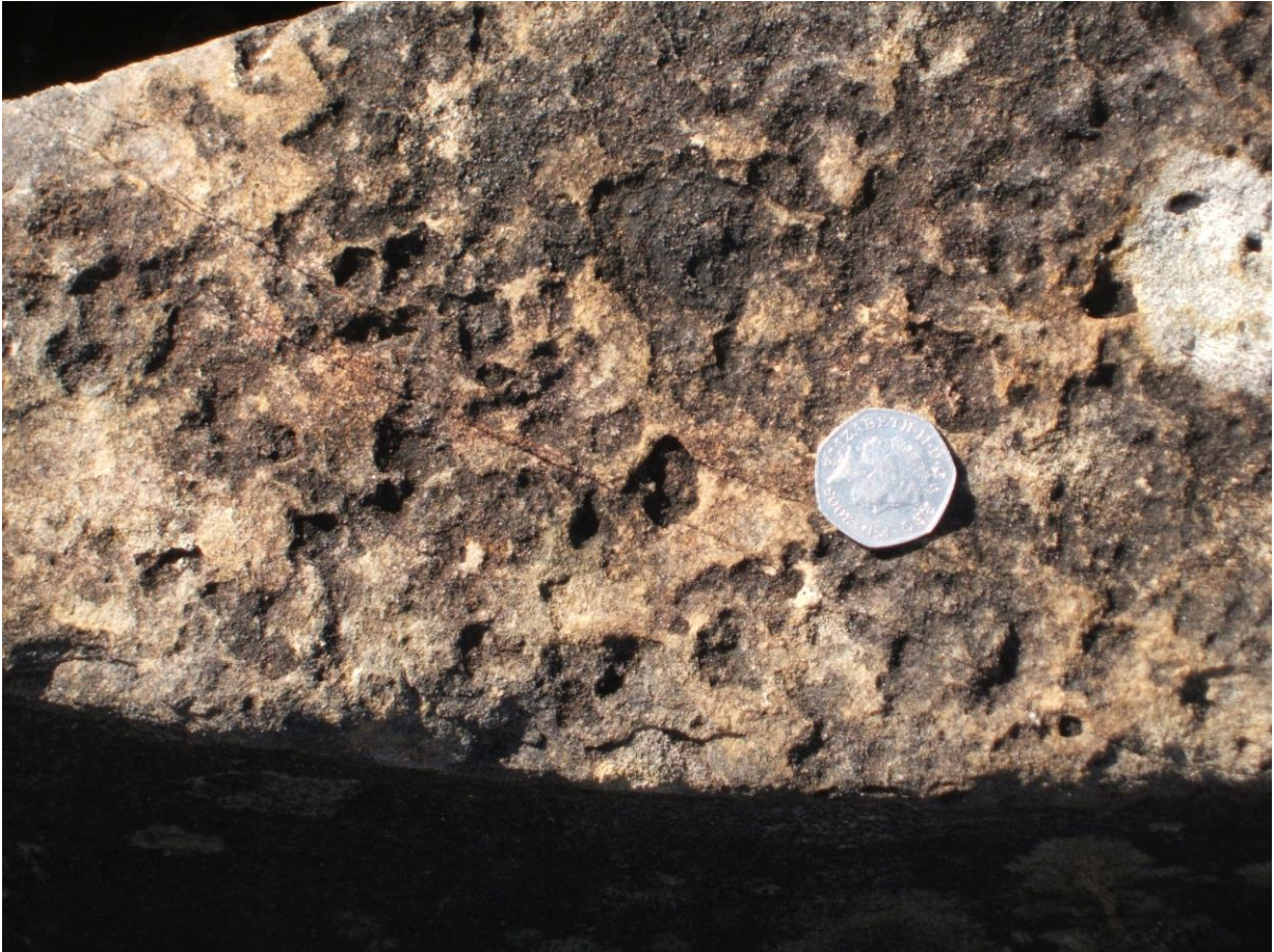
Photograph 3. Block of Honeycombed Sandstone showing distinctive carious weathering of calcareous sandstone
